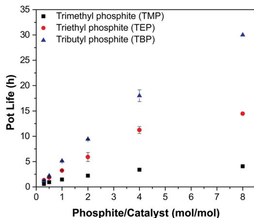
**Figure 2.** Effect of alkyl phosphite inhibitors on pot life of FROMP solutions (100 ppm GC2 complex). TBP exhibits the greatest pot life extension, followed by TEP, followed by TMP. Application of 8 equiv TBP to catalyst can increase pot life by >140×. Error bars are standard deviation;  $N = 3$ .
