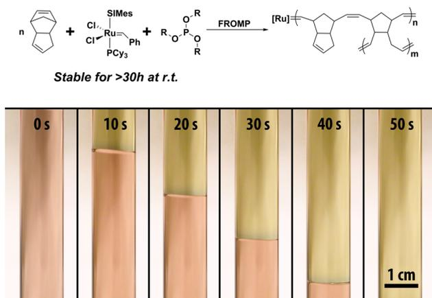
**Figure 1.** Scheme for phosphite-inhibited FROMP reaction. Inhibition of Grubbs' 2nd generation ruthenium catalyst (conc. = 100 ppm) by alkyl phosphites produces stable solutions with *endo*-DCPD for >30 h at r.t. that may be completely polymerized at any time via FROMP. The FROMP reaction shown here uses 0.5 equiv TBP to extend its pot life to >2 h, while maintaining a frontal velocity of ca. 7 cm/min.
