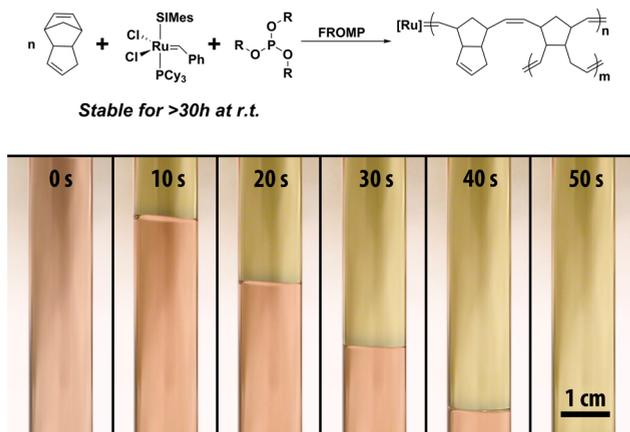
**Figure 1.** Scheme for phosphite-inhibited FROMP reaction. Inhibition of Grubbs' 2nd generation ruthenium catalyst (conc. = 100 ppm) by alkyl phosphites produces stable solutions with *endo*-DCPD for >30 h at r.t. that may be completely polymerized at any time via FROMP. The FROMP reaction shown here uses 0.5 equiv TBP to extend its pot life to >2 h, while maintaining a frontal velocity of ca. 7 cm/min.
