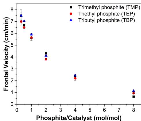
**Figure 3.** Effect of each alkyl phosphite on frontal velocity. While all tested phosphites slow frontal velocity, the effects are similar for all three compared to their disparate effect on in the pot life. Error bars are standard deviation;  $N = 3$ .
